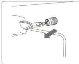
2: Unscrew the water inlet pipe from the back of the machine, pull out the filter screen with needle-nose pliers, clean it and reinstall it.
